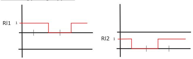
Confirmation of passage by pulse or "disk emulation" can be configured through the dipswitch Ds2  $n^{\circ}7$ ; if it is on, it will emulate the disk; if it is off, pulse will be generated when passing.
