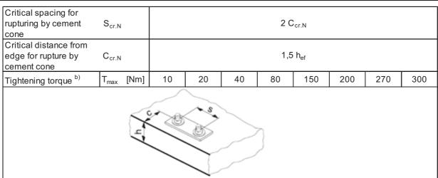
Estimate resistances must be reduced to distances from edge and spacing smaller than critical values.
