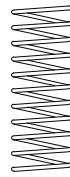
6010 Fail Lock Solenoid Spring These look the same as the fail open, but are actually much lighter in force Wire diameter is .032" This spring was also used on the 6100 Series Control Head.
