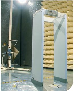
Exceptional immunity to environmental interferences makes the Metal Detector easy to use even when electrical noise is encountered.
