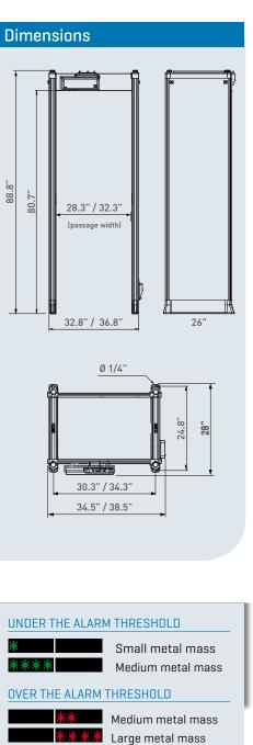
Green and Red Metering Signals Proportional to the Metal Mass Detected
