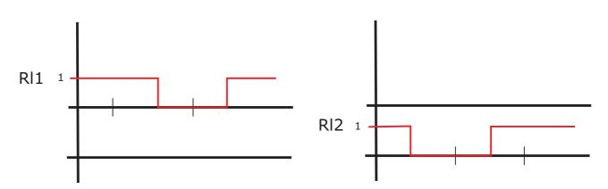
Confirmation of passage by pulse or "disk emulation" can be configured through the dipswitch Ds2 n°7; if it is on, it will emulate the disk; if it is off, pulse will be generated when passing.
