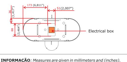
The distance between the boxes depends the size of the doors. Doors should be adjusted with a small gap between them of approximately 30mm. This gap is important to protect users.
