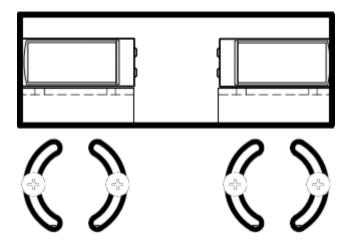
Loosening the screws holding the bracket to the panel will allow for some range of motion up and down.
