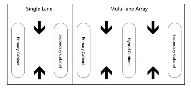
From the factory, each cabinet in an array is preconfigured to the requested operation and layout. Each lane has two directions of passage, each of which can be configured for controlled passage, free passage or no passage. This configuration can be changed in the field via settings on lane's logic controller located inside of the primary cabinet.
